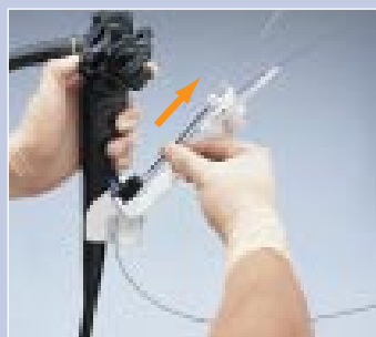
When the V-Marking is completely visible above instrument channel valve, raise the V-Groove forceps elevator.
